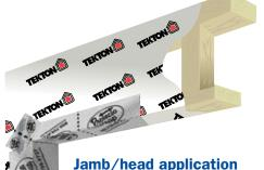
Cut 2 pieces of SUPER-STICK at 300mm\*. The tape is installed 150mm down the jamb & 150mm along the lintel at each of the top corners of the window or joinery opening. A 75mm wide by 150mm long sealing butterfly tape must be installed at 45 degrees across the corner of the head/jamb junction overlapping the corner by 3mm to create a seal at the corner junction.
