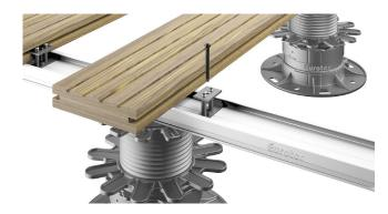
The Twin System Clip locks into the EVO substructure. The groove decking boards are fitted in place then secured with the stainless steel clamping plate. The Twin System Clip is ideal for composite decking.
