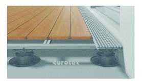
DrainTec profile offers an aesthetic finish to the perimeter of decks or simply run adjacent to the structure. The geometry prevents splashback from the deck staining the cladding.
