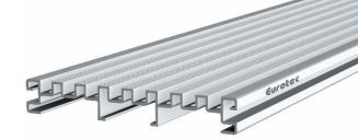
Its special geometry allows it to trap the rain so that the water falls directly onto the weatherproof layer, or into the gutter, without covering the door element or the façade cladding with reflected water (backsplash). Even heavy rain is drained in a controlled manner.
