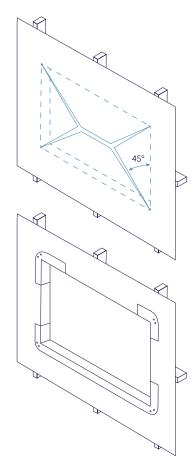
• Run the underlay over all joinery openings, these should remain covered until the joinery units are ready to be installed.
