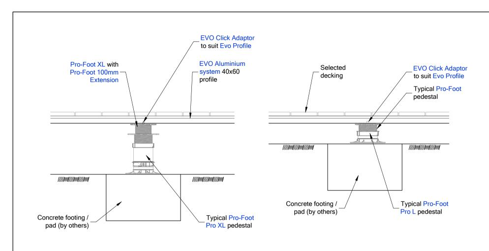
Typical Pro-Foot / EVO pedestal System on Spot Footings - Composite / Hardwood Decking
