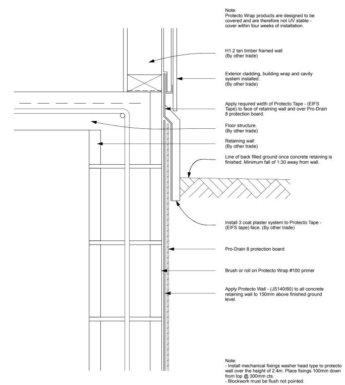
concrete retaining wall detail scale 1:5
