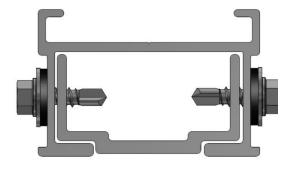
Profile joints of the substructure should always take place directly over a support point. To reduce vibrations, we recommend the adjustable feet every 2nd substructure profile around L / 2 offset to arrange.
